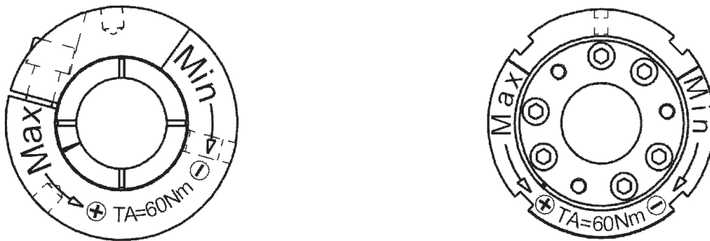
Marking of a safety coupling upon delivery (left: clamping ring; right: adjustment nut)
